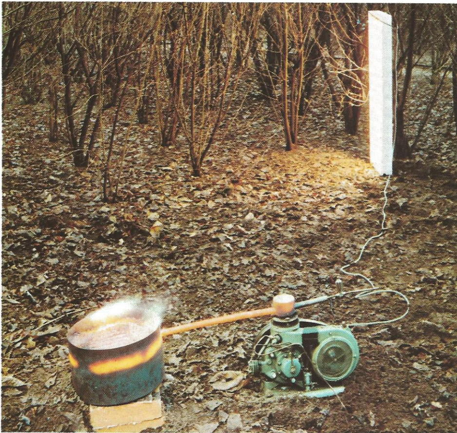
STIRLING ENGINES have an extraordinary ability to run on a wide range of fuels. The small research unit built by Philips in 1949, seen at right driving a 200W generator supplying a battery of fluorescent lamps, runs on air heated by a coal fire seen burning in the open brazier. The later unit below is mounted on a portable frame together with ten fuel containers, any of which can be switched in while the engine is running. The output of 7.5 kW at 3000 r.p.m. is maintained on supplies as diverse as diesel fuel, crude oil, alcohol or salad oil
