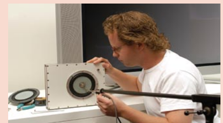
Measuring on a Bass loudspeaker unit.
